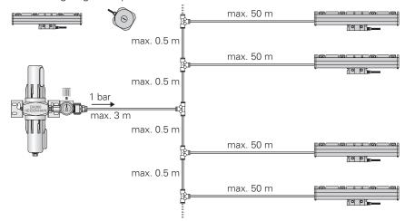
Max. tubing lengths for serial encoder connection
