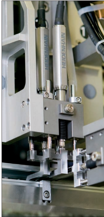
Testing station for flatness inspection
