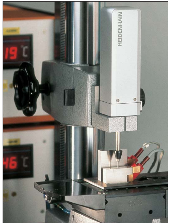
Thickness gauging of silicon wafers
