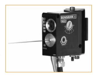
The unique tool recognition electronics determine whether a tool is present by analysing the reflective light pattern from the rotating tool. Random light patterns created by coolant and swarf are ignored, reducing the chances of not detecting a broken tool due to coolant blocking the beam.
