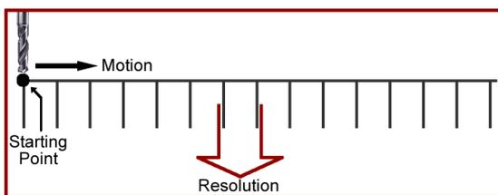
example, in a ball-screw-based positioning system, a theoretical resolution of 1μm can be obtained by combining a 10mm/rev screw, a 1000-line encoder, and a x10 multiplier. The actual motion system will never be able to make a single 1μm step due to friction, windup, and mechanical compliance. Therefore, the practical resolution is actually less.
