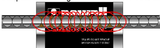
This field interacts with the nickel chrome elements contained in the scale. A set of four pickup coils detect variations in the induced field that are then combined and processed by the electronic circuitry to generate a signal that varies as the head moves along the scale. Depending on the position of the reader head as it passes over each element, the phase shift of this pickup signal relative to the drive signal will vary between 0 and 360 degrees.
