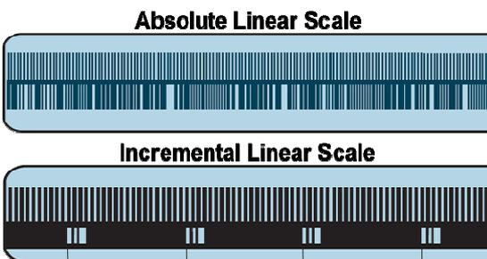
In some cases this may necessitate machine movement over large lengths of the measuring range. To speed and simplify such “homing sequences,” some scales feature distance-coded reference marks—multiple reference marks that are individually spaced according to a mathematical algorithm. The subsequent
