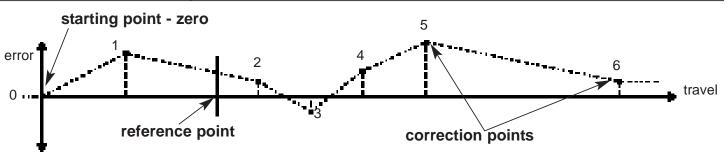
The scale travel is broken down into a number of user-defined segments, each with its own correction factor, measured against an high-accuracy standard. The following parameters need to be identified:
