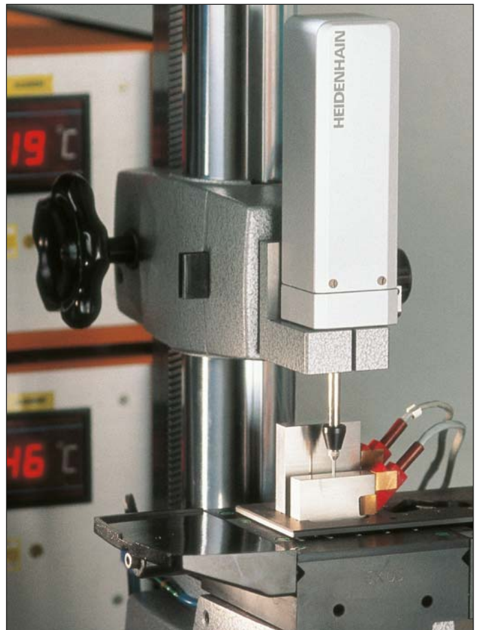
Calibration of gauge blocks
