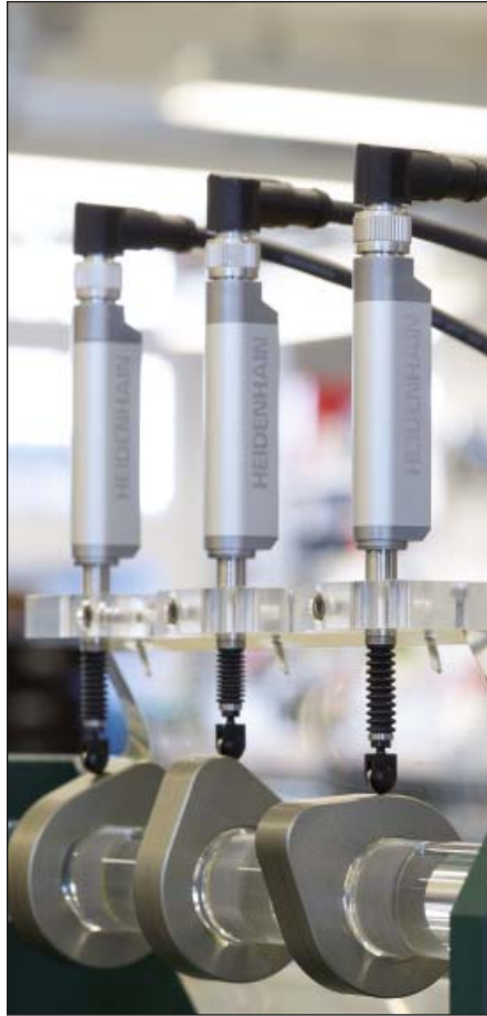
Testing station for flatness inspection
