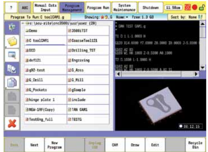
Graphic preview of part program in Program Management with estimated run time.
