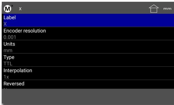
Specify the signal type, encoder resolution, and direction for the encoder being configured. Verify that the encoder displacement and direction of travel are correct using some know standard of size and observing the major directions for part coordinates relative to the measuring image of the system.
