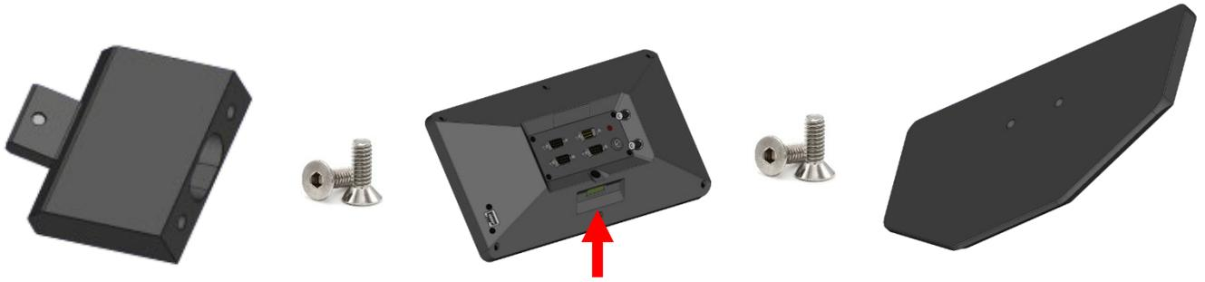
Using a 3MM Allen wrench and the supplied M6 screw, connect the riser block to the opening on the rear panel of the Mx100.
