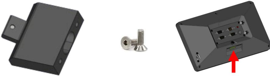
Using a 3MM Allen wrench and the supplied M6 screw, connect the riser block to the opening on the rear panel of the Mx100. The hole spacing is 38MM with a ¼"-20 thread pattern. Screws required to connect the OEM mount to the machine mount are not included in the Mx100 mounting kit.
