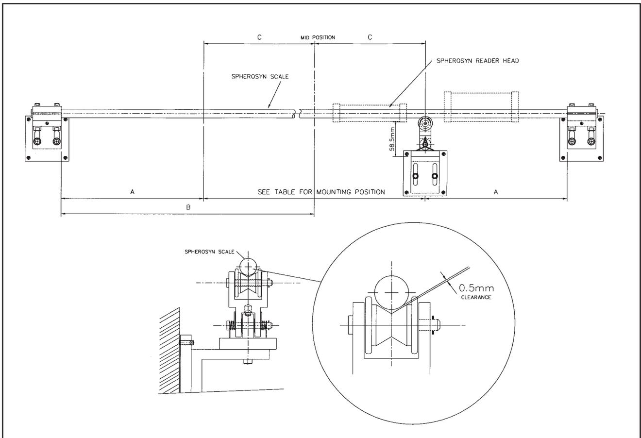
**Figure 5.6 - Spherosyn Long Scale Mounting and Support Details**
