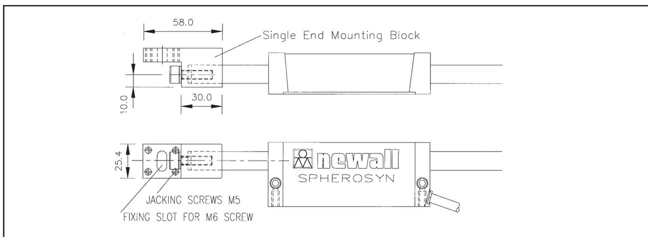
**Figure 5.4 - Spherosyn Single End Mounting**
