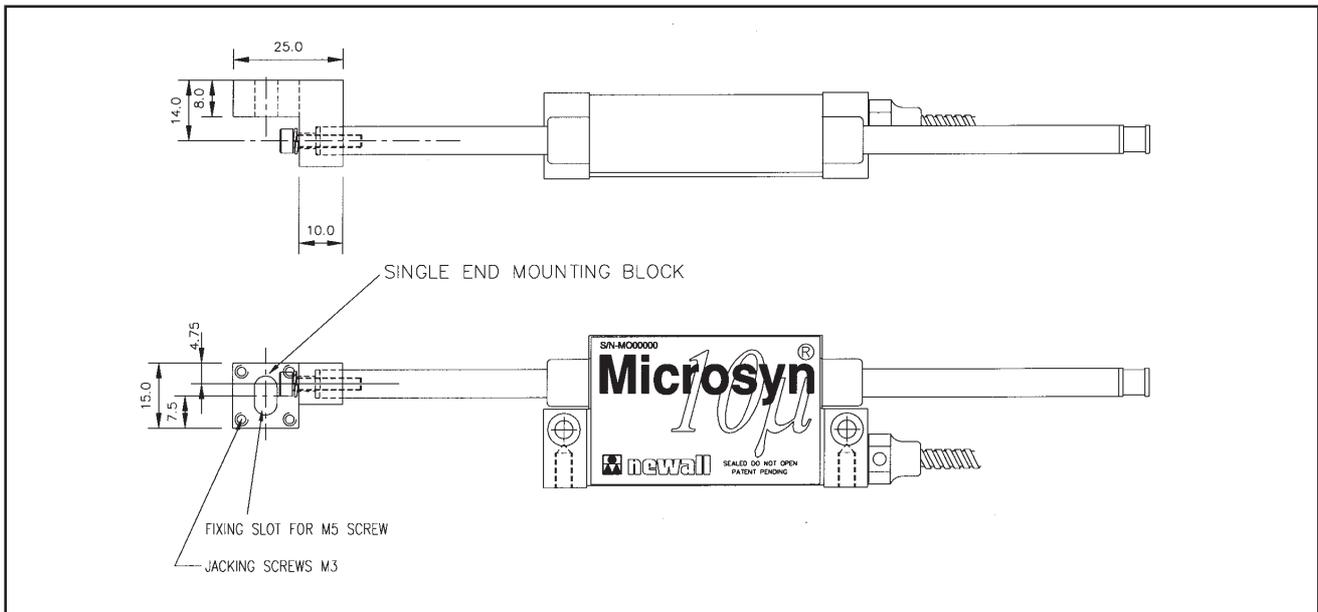
Figure 5.10 - Microsyn Single End Mounting
