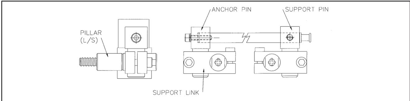
**Figure 5.8 - Microsyn Scale Support Bracket**
