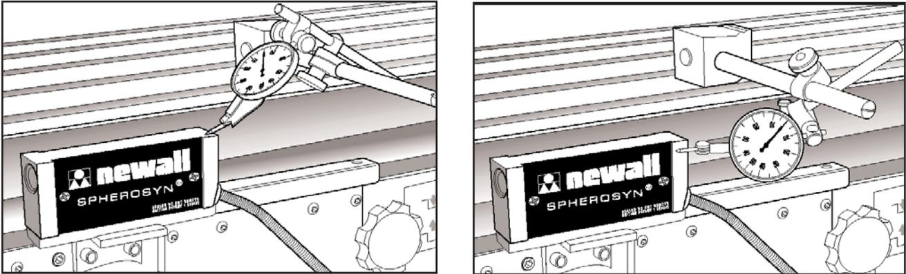
*Figure 4.1 - Alignment of the Spherosyn Reader Head*
