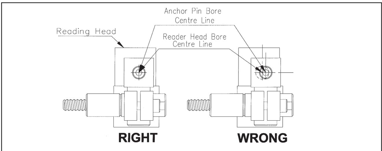
**Figure 5.9 - Reader Head and Bracket Alignment**
