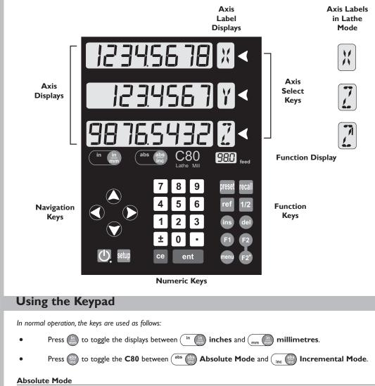
In this mode, the C80 will display the positions of the three axes relative to a fixed datum.
