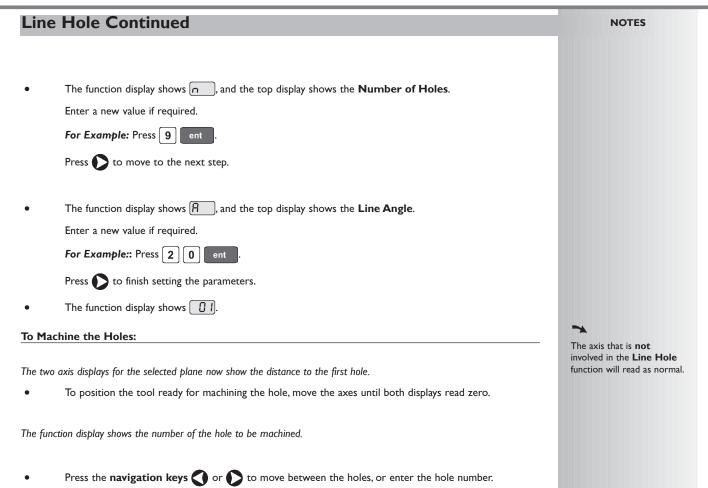
• When all holes have been machined, press (F1) or (F2) to turn the function off.
