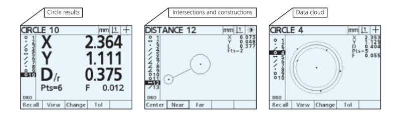
**Optical edge detection** Achieve higher throughput, more accurate measurements, and more consistent data with optical comparators using optical edge detection. Automatic point entry reduces operator subjectivity and fatigue.
