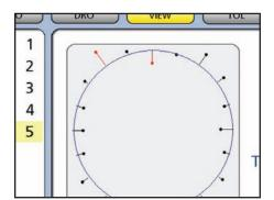
**Results view** Graphic representation of the data cloud with errors. Feature measurement results and fit type.
