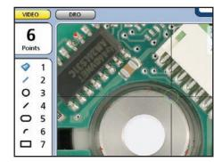
**Automatic Video Edge Detection** For improved throughput and accuracy.
