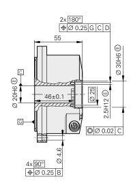
Shaft coupling with ring nut
