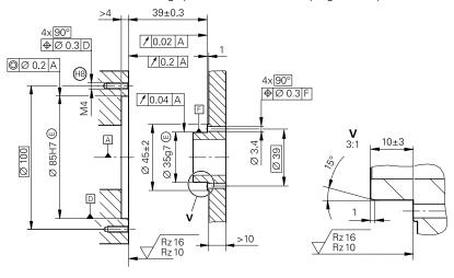
Alternative mounting option: Front-end shaft coupling with positive lock (for more dimensions, see option without positive lock)
