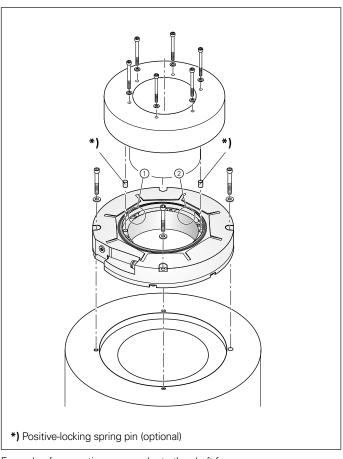
Example of connecting an encoder to the shaft face
