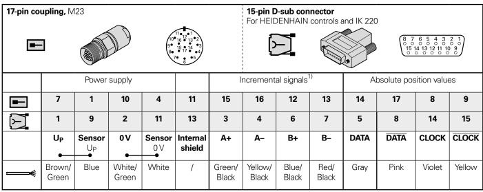
Cable shield connected to housing;  $U_P$  = Power supply voltage
