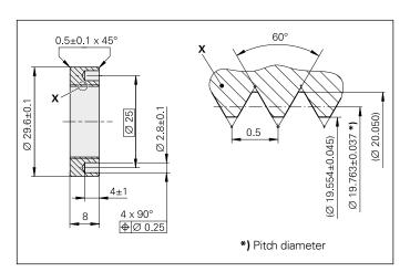
Ring nut for hollow shaft Ø 20 mm
