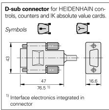
The pins on connectors are **numbered** in the direction opposite to those on couplings or flange sockets, regardless of whether the connecting elements have
