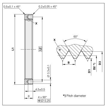
Ring nut for hollow shaft Ø 35 mm Ø 50 mm Ø 60 mm Ø 100 mm
