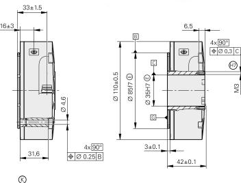
Shaft coupling with ring nut
