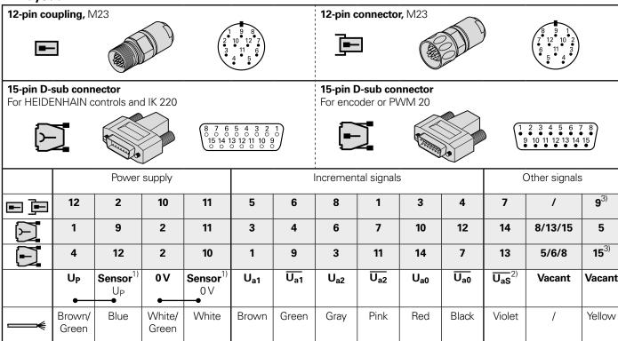
Cable shield connected to housing; UP = Power supply voltage
