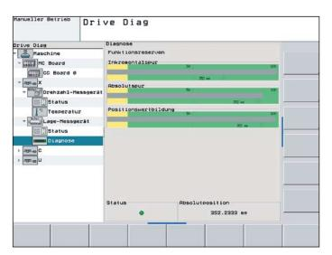
Diagnostics in the control loop on HEIDENHAIN controls with display of the valuation number or the analog encoder signals
