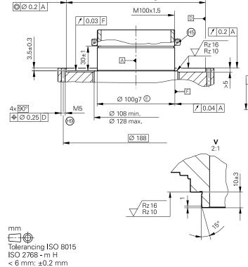
Ø 118 min. Ø 128 max. Ø 114.7±0.1 Ø 106 6x 60° ⊕ Ø 0.25 E Ø 4.5 8.5 / 0.2 A 28.2±0.3 w 🖡 / 0.03 A Ø 100g7 🖲 / 0.04 A A-2 4x 90° M5 D Ø 180H7 🖲 ф Ø 0.25 D (19) Ø 188 Ø Ø 0.2 **(K)** Alternative mounting option: Front-end shaft coupling with positive lock (for more dimensions, see option without positive
