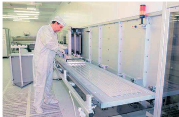
Vacuum machine for application of chromium layers
