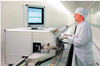
30 m long measuring machine for scale tapes
