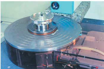
Angle comparator, measuring step approx. 0.001°
