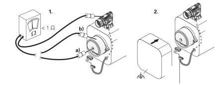
Clamp (when present) must be screwed to the motor housing so as to be conductive.
