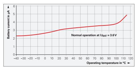
EBI 1135/135: typical discharge current during normal operation (U<sub>B</sub> = 3.6 V)
