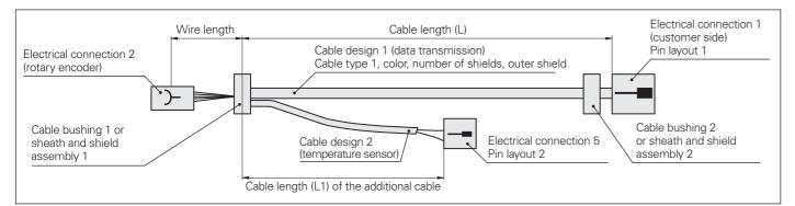
Temperature sensor signals via rotary encoder PCBA
