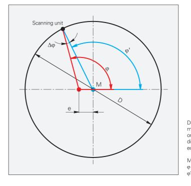
Resultant measuring error  $\Delta \phi$  for various eccentricity values e as a function of the mean graduation diameter D
