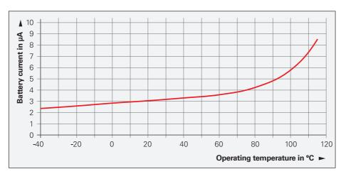
EBI 4010: typical discharge current during normal operation (U<sub>BAT</sub> = 3.6 V)
