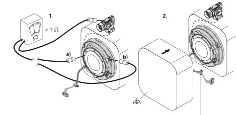
Clamp must be screwed to the motor housing so as to be conductive.
