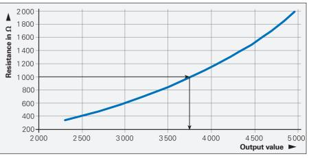
Example for the KTY 84-130 temperature sensor: which is equal to 375.1 K or 102 °C.
