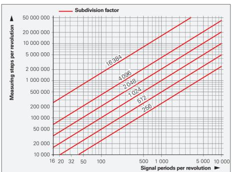
Signal periods per revolution and the resulting number of measuring steps per revolution as a function of the subdivision factor
