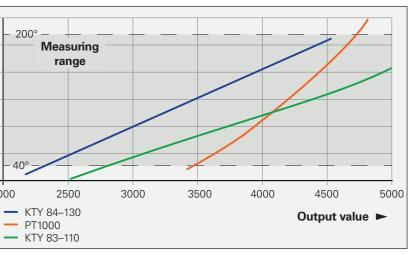
Figure 2: Relationship between the output value and the temperature value using the example of the
