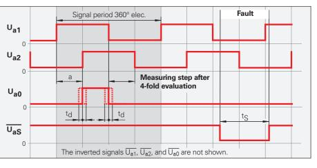
The distance between two successive edges of the incremental signals U<sub>a1</sub> and U<sub>a2</sub> through 1-fold, 2-fold, or 4-fold evaluation is one measuring step.
