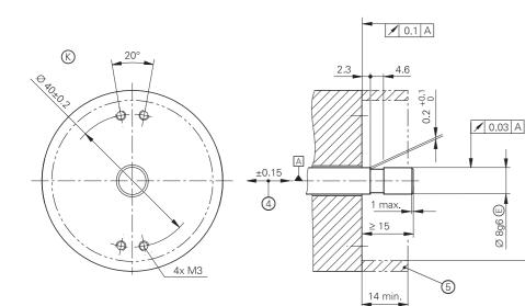
mm Tolerancing ISO 8015 ISO 2768 - m H < 6 mm: ±0.2 mm
