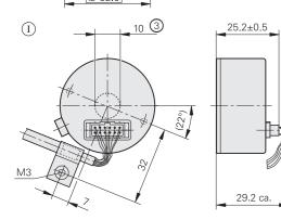
Axial PCB connector and round cable
