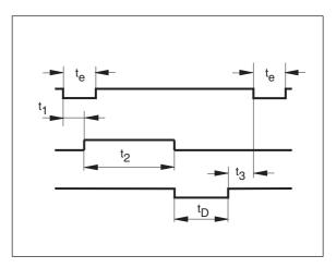
Next possible signal for measured value output:  $tE = t_1 + t_2 + t_D + t_3 [s]$
